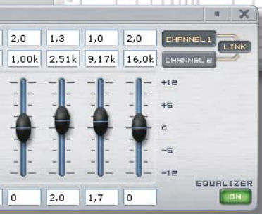
Equaliser module with graph 10 bands per channel, frequency and Q factor selected as required. Excellent graphic view of your work on the EQ.
