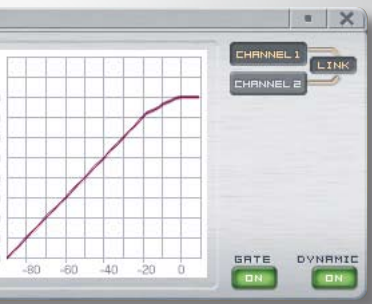
Dynamic module System compressor, limiter and noise gate with all necessary setting options.
