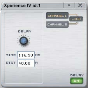
Delay module For delaying the speaker system (DelayLine applications). Settings in milliseconds or metres.
