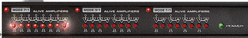
AX16 switches to backup amplifier
