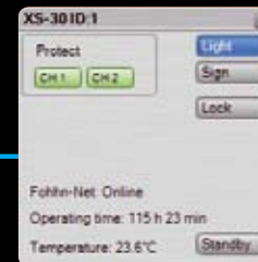
Status module Displays the temperature and operating time. Protection. Lock function. Signal function = display flashes indicating that the device is detected. Sinus tone and pink noise generator.
