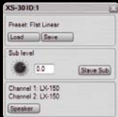
Preset module Select sound presets and speaker presets. Sub level adjustment.
