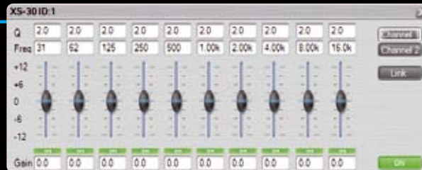
Parametric equaliser module with graph 10 band parametric EQ, frequency and Q factor selected as required. Excellent graphic view of your work on the EQ.
