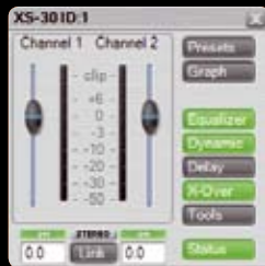
Main module Individual audio devices or presets are selected with one mouse click. Adjustment of volume level, channel on/off and stereo/mono mode.
