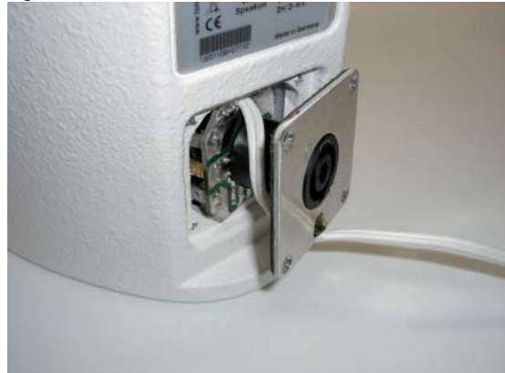
4. Thread the speaker connecting cables through the bottom cable recess and attach the connection terminal back to the speaker housing.
