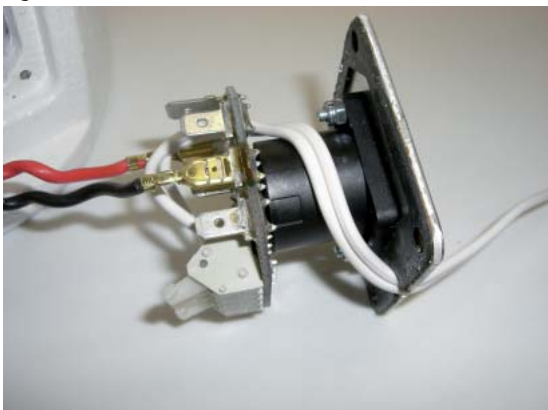
3. Clamp the speaker connecting cables to the 4-way terminal strip
