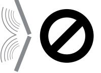
IMPORTANT: NEVER INSTALL 2 OR MORE AX12C AIMING THE SPEAKERS TO EACH OTHER WITH CLOSED ANGLES. In other words, NEVER use the 4° STACK position between two speakers.
