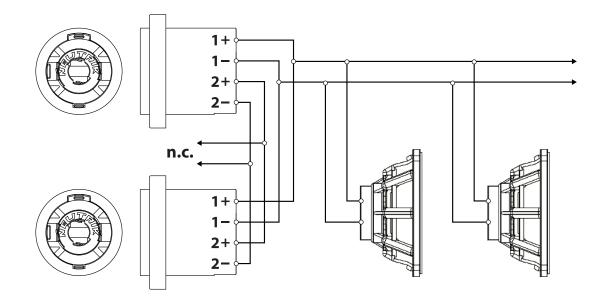
WARNING: the maximum quantity of AX12C that can be linked together depends by the load capacity of the appropriate processed amplifier. When powered from the SW2100A subwoofer or from the QC2.4 suggested amplifier, a maximum of four AX12C can be connected to each power output.
