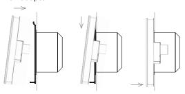
Carefully tighten the fixing screw to fix touch panel on the wall.
