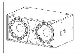
The 10" low frequency transducers are equipped with waterproof cones and this feature, together with the moisture resistant cabinet, makes the SW210P suitable for use in light duty outdoor applications. The transducer technology combines a 3" sandwich voice coil with a fiberglass former progressive wave Konex spider; a cloth surround with DAR technology; a high excursion ferrite magnet circuit with demodulating ring; and a ventilated voice coil and magnet to reduce power compression.
