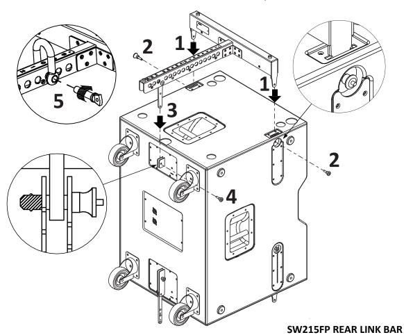
When lifting the system always proceed gradually step by step, paying attention to secure the fly bar to the box (and the box to the other boxes) before pulling up the system: this makes easier to insert properly the locking pins. Also when the system is released down, unlock gradually the pins.
