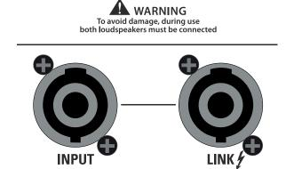
**LINK** - Power output in parallel with the INPUT socket for connecting the unit to another speaker. The number of SW215P cabinets that can be connected in parallel depends on the amplifier load capacity.
