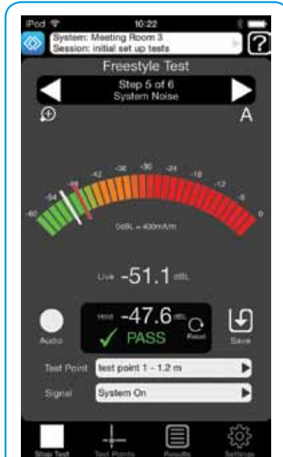
System Noise test Test with system ON.
