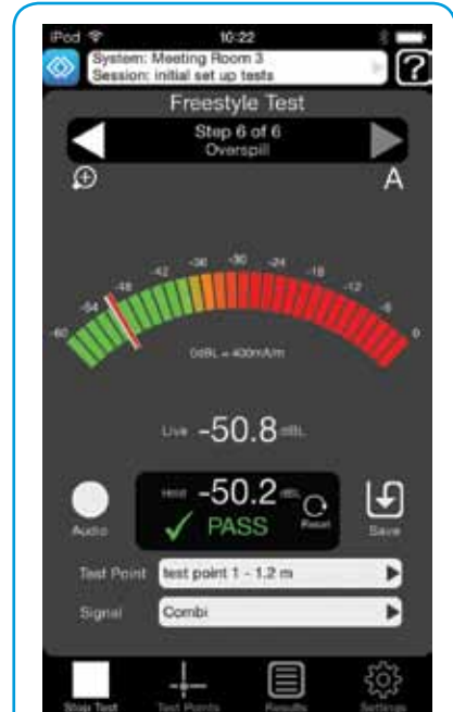
Overspill Test room overspill with COMBI signal.
