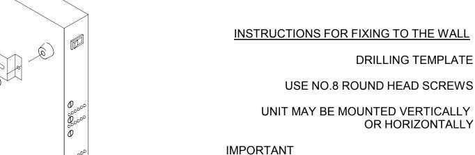
USE 4 WALL FASTENERS, EACH CAPABLE OF SUPPORTING 6.35kg / 14lb, TO PROVIDE A SAFETY FACTOR OF 4. USE APPROPRIATE FIXINGS, PLUGS OR ANCHORS, FOR THE TYPE OF WALL THE UNIT IS TO BE MOUNTED ON.
