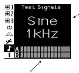
Loop Current bar graph for each channel. Shows Loop output current in 2dB steps from >-20dB to 0dB in green. Red = clipping Test signal selected by rotary control:
