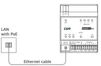
The integrated IEEE 802.3af PoE support allows installation in areas where PoE network infrastructure is installed.
