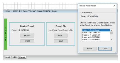
**PRESET:** you can store or recall preset in the device's memory or load and save presets in your computer HD as \*.pcf files. **Note:** the user preset no. 4-U can be reloaded also from the unit's control panel without the need to re-connect to the pc.
