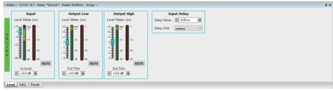
Input - Level: adjusts the input level gain in the range of -30 ÷ +6 dB (this is a digital control after the A/D converter).
