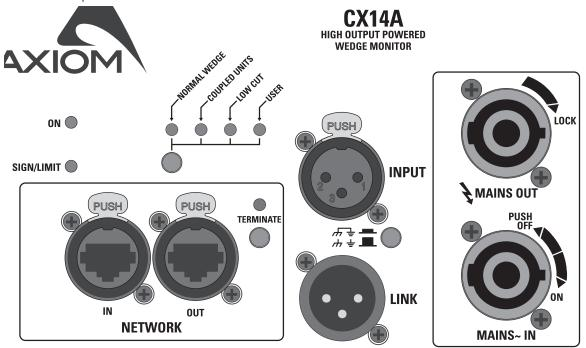
**INPUT** - Audio signal input with locking XLR connector. It has a fully electronically balanced circuitry including AD conversion for the best S/N ratio and input headroom.
