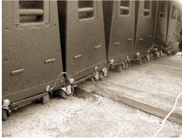
Figure 5.3: Array prepared on a uneven ground
