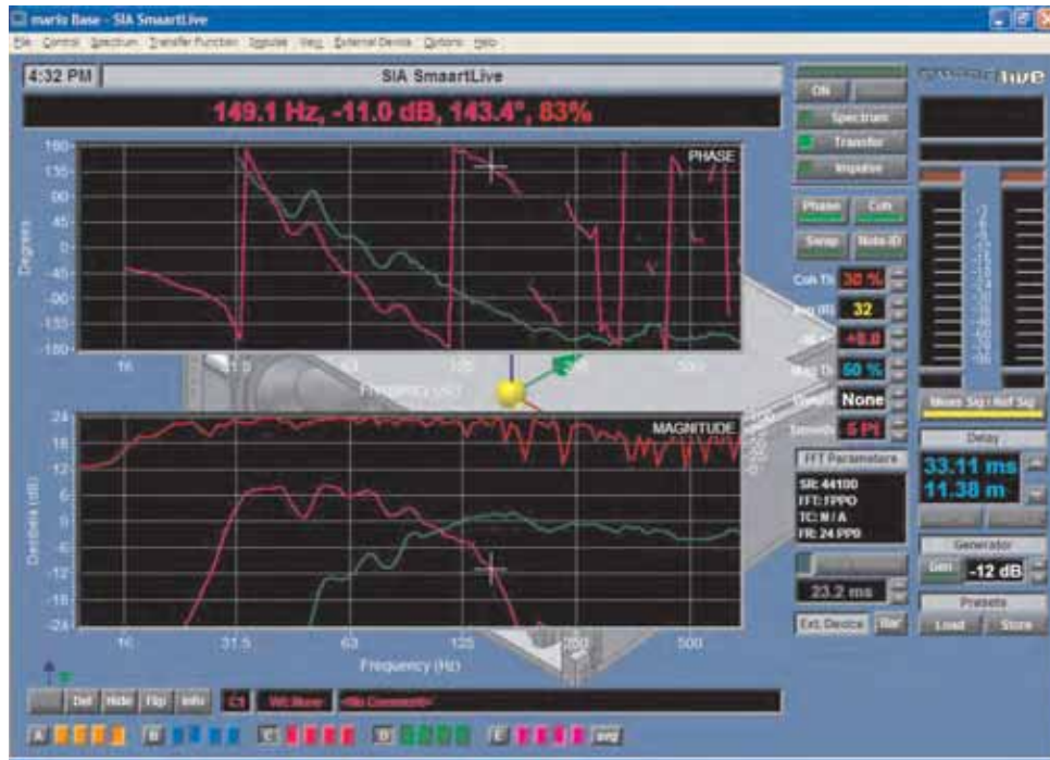
Figure 6.6: Delay adjustment, SUB signal lags in phase.
