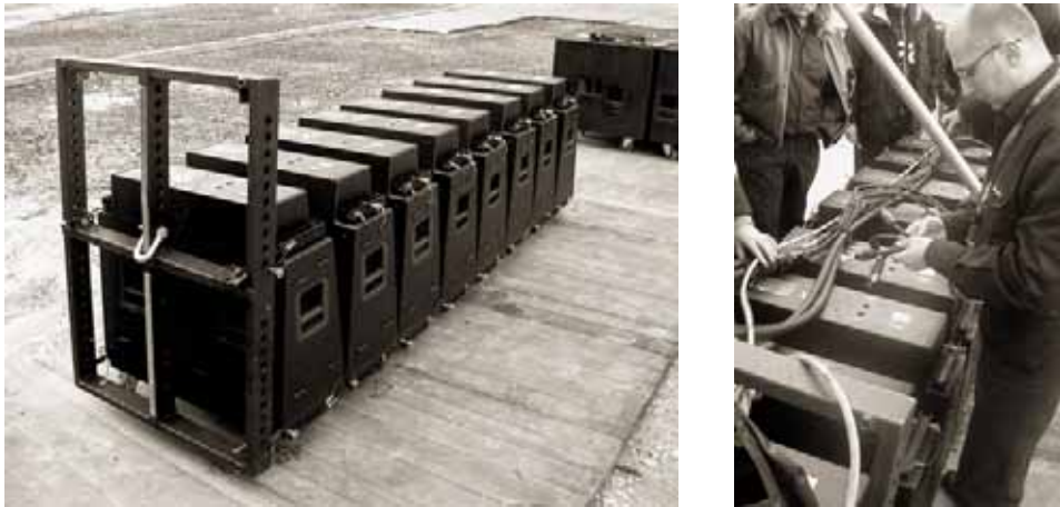
Figure 5.5: Array coupled in the front and ready (on the left) and power wiring (on the right).
