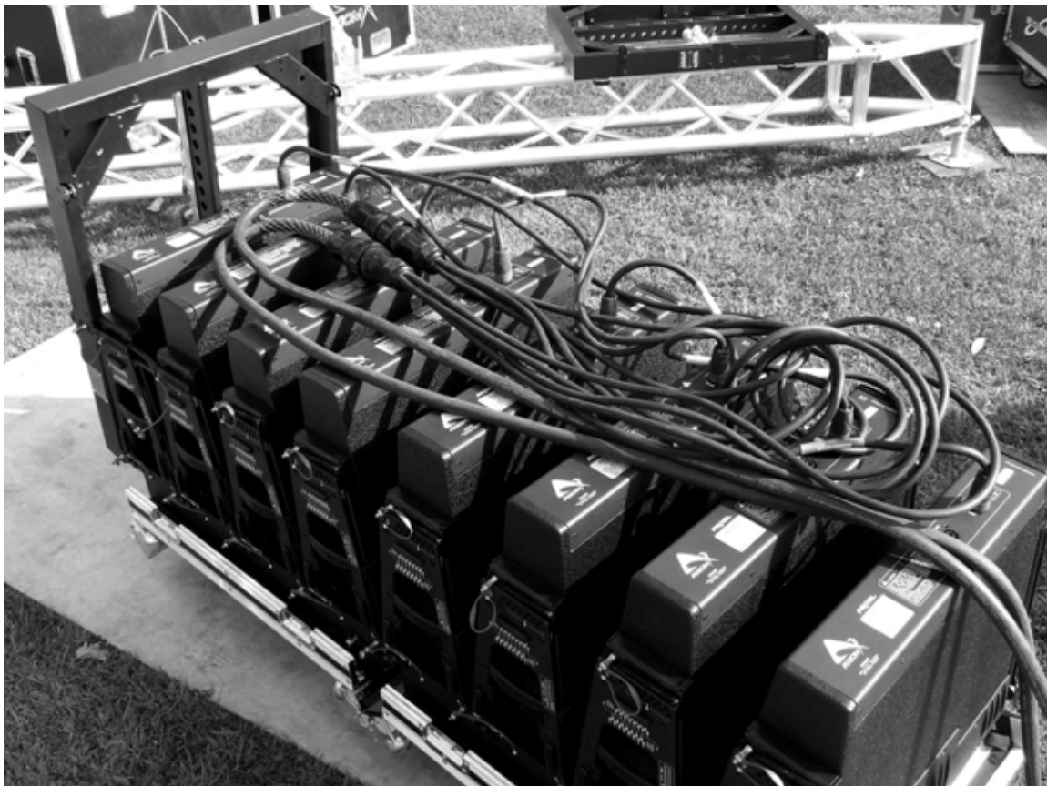
Figure 5.20: AX2265P array coupled in the front and power wired ready to lift
