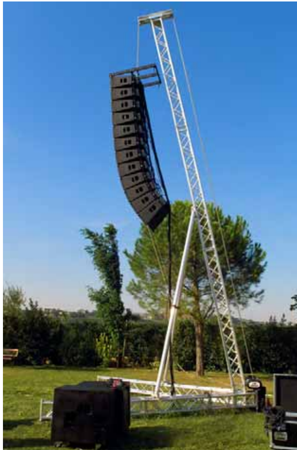
Figure 3.3: PLFTMQD30 9.5m tower with 600 kg capacity.
