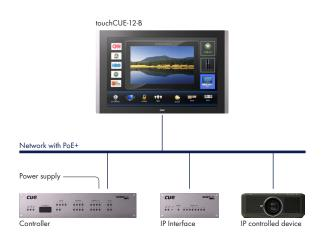
The following diagram describes the use of touch panel with IP interfaces only. This configuration allows to create cost effective distributed control solution where touch panel serves as controller and graphic user interface in one box. In Cue Visual Composer touch panels and controllers are programmed in the same way, which makes possible to use touch panels as fully functional control units.
