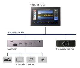
The following diagram describes the use of touch panel with IP interfaces only. This configuration allows to create cost effective distributed control solution where touch panel serves as controller and graphic user interface in one box. In Cue Visual Composer touch panels and controllers are programmed in the same way, which makes possible to use touch panels as fully functional control units.
