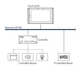
The following diagram describes the use of touch panel with IP interfaces only. This configuration allows to create cost effective distributed control solution where touch panel serves as controller and graphic user interface in one box. In Cue Visual Composer touch panels and controllers are programmed in the same way, which makes possible to use touch panels as fully functional control units.
