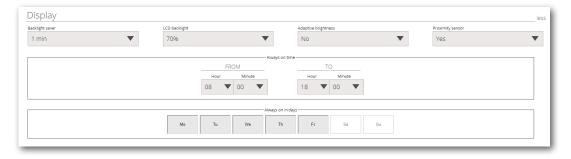
In "Backlight saver" you can set after how long the display illumination is turned off in case of panel inactivity. The default setting is "1 min".
