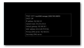
In the default setting, the unit is enabled to get the IP address and DNS servers using the DHCP of your network. Check whether the IP address, gateway and DNS servers correspond to your network. In the "DHCP" item you can check whether the IP address has been acquired through DHCP (On) or not (Off). If the setting is not suitable for you, it can be changed later - for description how to do this see the chapter Basic configuration of the touchONE-manager unit - IP Settings.
