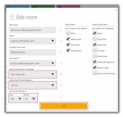
In the item "Require confirmation of meetings", activate the function by selecting "By dialogue box on the panel", "By occupancy sensors" or "By occupancy sensors or dialog box". If you do not require confirmation, choose "Not required ". The default setting is "Not Required ".
