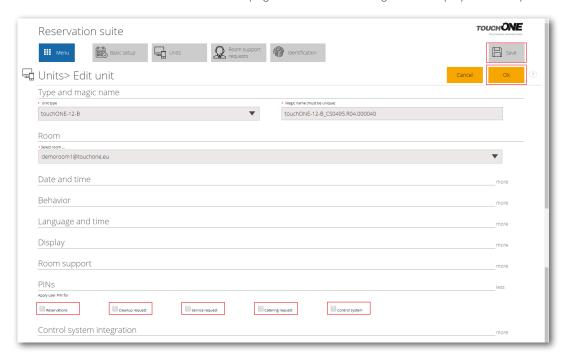
Using checkboxes in the section "PINs / Apply user PIN for", you can state which functions will require the entering of PIN on the given panel:
