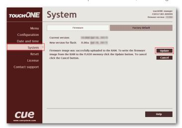
The firmware upgrade takes about one minute and then the unit restarts. Do not shut down or disconnect the power (LAN) during the update, as this might damage the unit. If upgrade has been successful, the following screen will come up.
