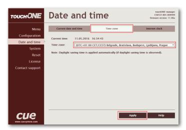
The touchONE-manager unit requires automatic synchronization of its clock with the internet (NTP) servers. If you want to change the setting of the internet time servers, select "Internet clock". Here you can change the names or IP addresses of the primary NTP server and the secondary NTP server. The default setting of the servers is "time.nist.gov" and "tak.cesnet.cz". Be sure to click the "Apply" button for any changes to become effective.
