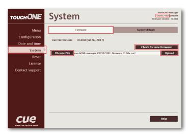
After the file with new firmware is uploaded into the unit, the following screen will come up. Apply new firmware by clicking "Update".
