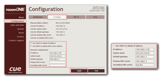
In changing the IP settings, you need to reset the touchONE-manager unit. Confirm the changes in the setup by clicking "Yes" on the next page. This will also initiate the reset.
