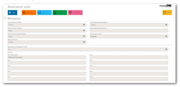
The items "Minimum duration of meeting" and "Maximum duration of meeting" allow you to set the limits for reservations made through a panel. The maximal duration is limited to the midnight of the given day. Default setting for the minimum time is 15 minutes and "None" for the maximum time. The item "Maximum duration of extended meeting" allows you to limit the maximum length of meeting extended by means of the panel. The default value is "None", lasting until the end of the day at maximum.
