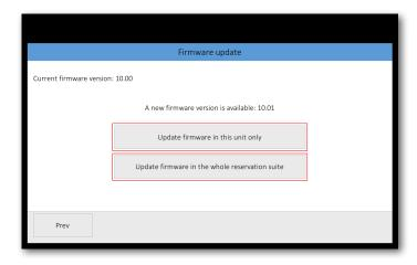
Firmware update takes approximately 1 minute and then the unit is restarted. Do not shut down or disconnect the power (LAN) during the update, as this might damage the unit.
