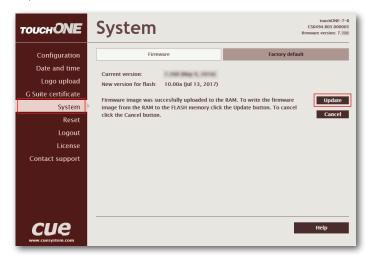
The firmware upgrade takes about one minute and then the panel restarts. Do not shut down or disconnect the power (LAN) during the update, as this might damage the unit. If upgrade has been successful, the following screen will come up.
