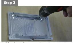
Drill four holes for screws. Use indicated pre-drilled positions.
