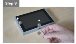
Loosen the fixing screw using delivered Allen key - 1 and remove back cover of the panel - 2, 3.
