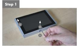
Loosen the fixing screw using delivered Allen key - 1 and remove back cover of the panel - 2, 3.
