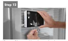
Connect Ethernet cable to the panel and put the panel on the back cover - 1, 2. Carefully tighten the fixing screw to fix panel on the back cover - 3.
