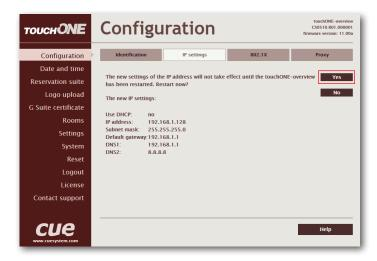
If your LAN is secured using 802.1X, select the "802.1X" tab at the top. Supported authentication methods are MD5 and TLS.
