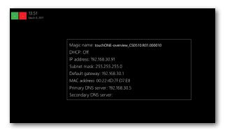
In the "IP address" line, the current IP address is shown. Run the Internet browser on your PC and type in the touchONE-overview unit IP address.
