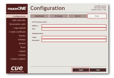
Enter Address and Port of the proxy server. If the proxy server requires authentication, enter the credentials for the proxy server in "Login" and "Password". Click "Apply" to save the changes.
